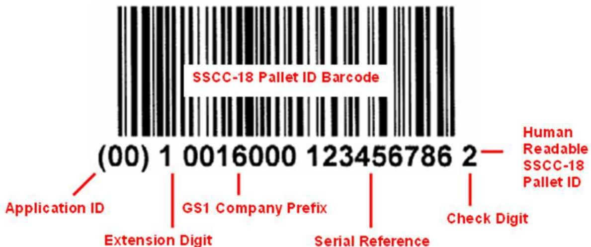
Below is a GS1 example of an SSCC18 pallet label that includes human readable information as well as additional bar codes. Such labels are acceptable for General Mills purposes so long as the SSCC18 pallet label is visible, scan-able, and positioned as the top or bottom bar code (avoid any middle position for an SSCC18 pallet label bar code).
